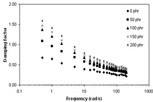
**Figure 3** Damping factor as a function of frequency of NR compounds filled with various FA loadings
