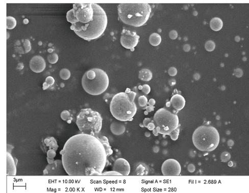
**Figure 1** SEM micrograph of FA particles used in the present study
