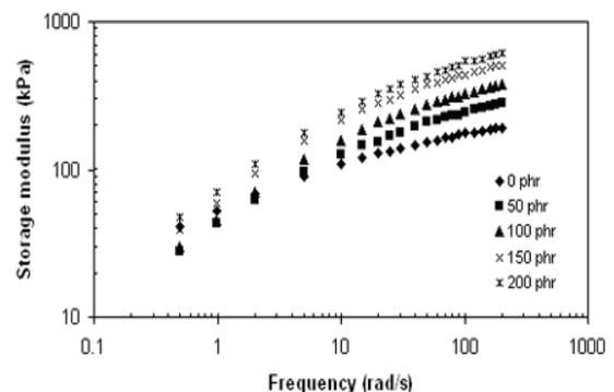
**Figure 2** Storage modulus (G') as a function of frequency at 7 % strain of NR compounds filled with various FA loadings
