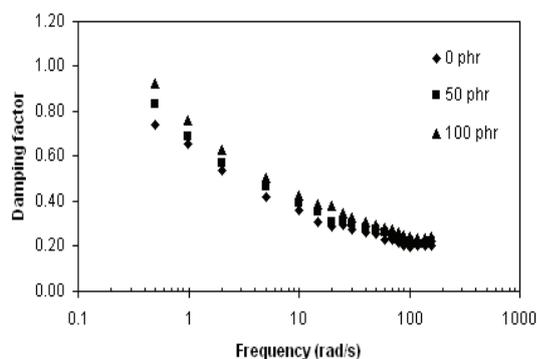
**Figure 4.** Damping factor as a function of frequency of IR compounds filled with various FA loadings
