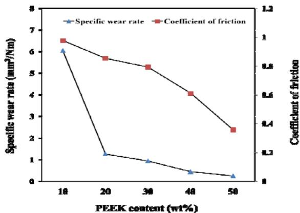
**Figure 5.** Variations in coefficient of friction and specific wear rate as a function of PEEK content (test condition: load 1N, sliding speed 0.1 m/s).
