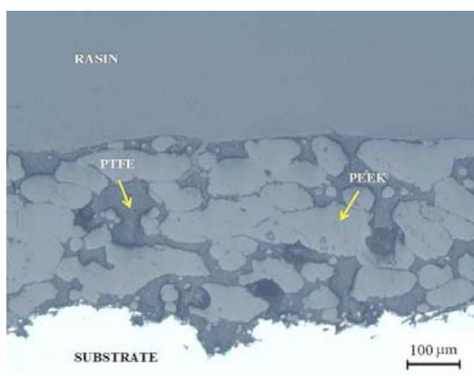
**Figure 1.** Cross sectional view of the PTFE composite coating with 50 wt% PEEK contents.
