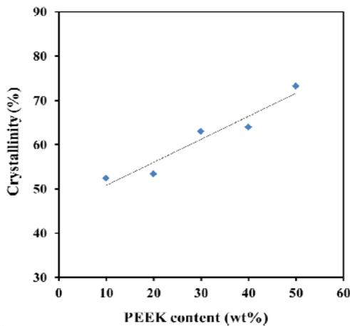
**Figure 4.** The effect of PEEK content on crystallinity of PEEK/PTFE composite coatings.
