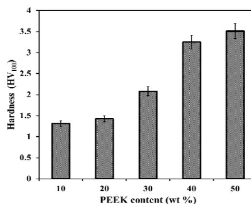
**Figure 3.** The effect of PEEK content on hardness of PEEK/PTFE composite coatings.
