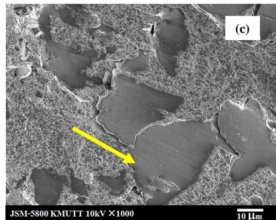
**Figure 6.** Worn surfaces of the PEEK/PTFE composite coatings (a) 30 wt%, (b) 40 wt% and (c) 50 wt% of PEEK (test condition: load 1N, sliding speed 0.1 m/s).
