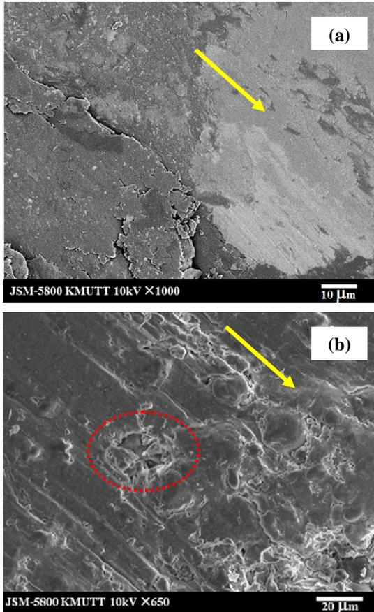
**Figure 7.** Worn surfaces of the PEEK/PTFE composite coatings with 50 wt% of PEEK after testing with different load (a) 1 N and (b) 3 N.
