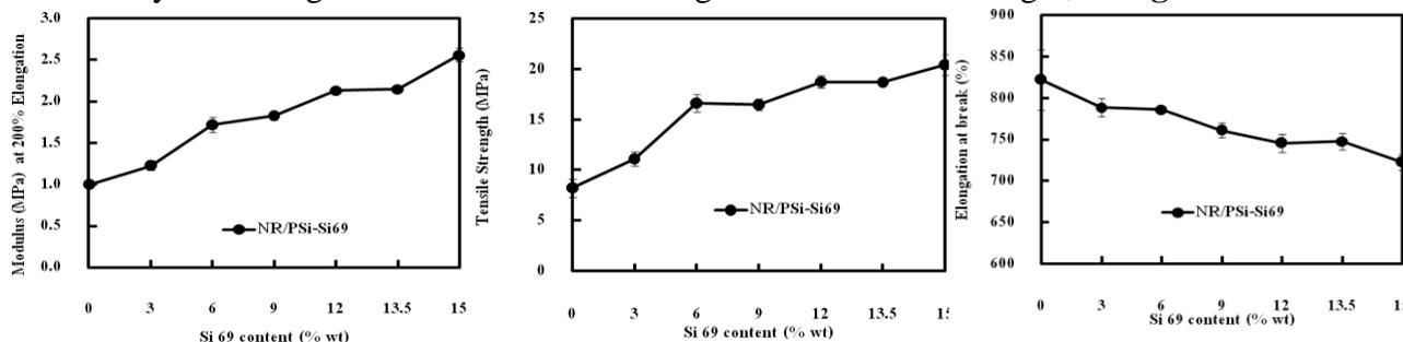
**Figure 3** Modulus at 200 % elongation (a), tensile strength (b) and elongation at break (c) of Si-69 modified PSi/NR vulcanizates.
