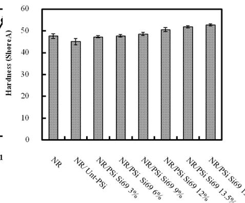
**Figure 6** Hardness of Si69 modified PSi/NR vulcanizates.
