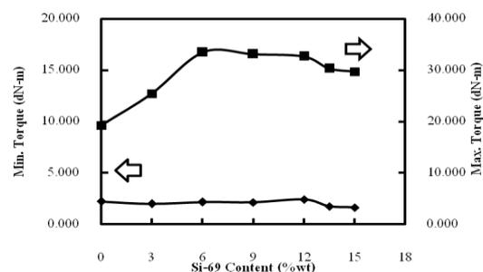
**Figure 2** Minimum and Maximum torques of Si-69 modified PSi/NR compound.
