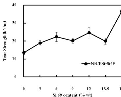
**Figure 4** Tear strength of Si69 modified PSi/NR vulcanizates.
