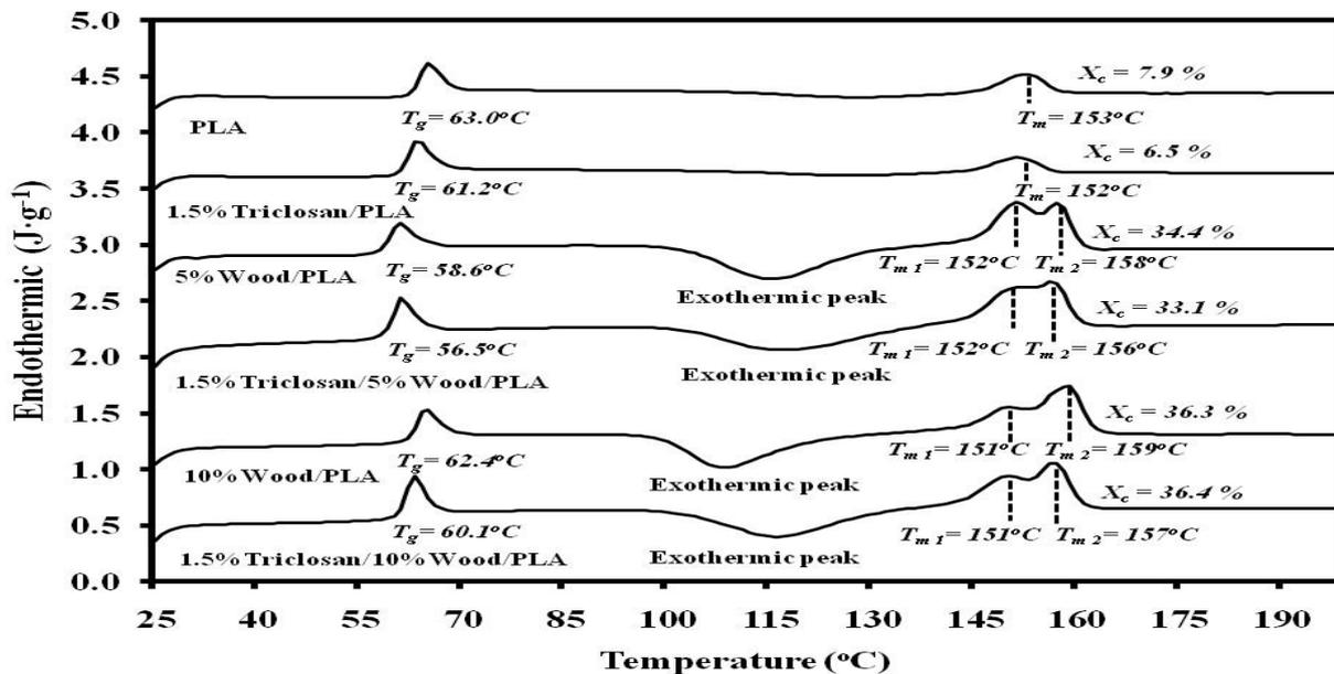
Figure 1. DSC curves for PLA, wood flour/PLA, triclosan/PLA and triclosan/wood flour/PLA
