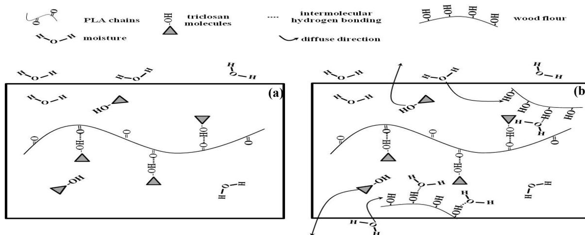
**Figure 2.** A possible model of moisture regain by wood in triclosan/PLAs:(a) no wood; (b) with wood.
