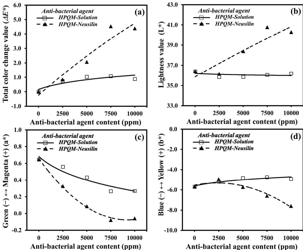
**Figure 2** Color changes of PP samples added with HPQM: where (a)  $\Delta E^*$  value, (b)  $L^*$  value, (c)  $a^*$  value and (d)  $b^*$  value
