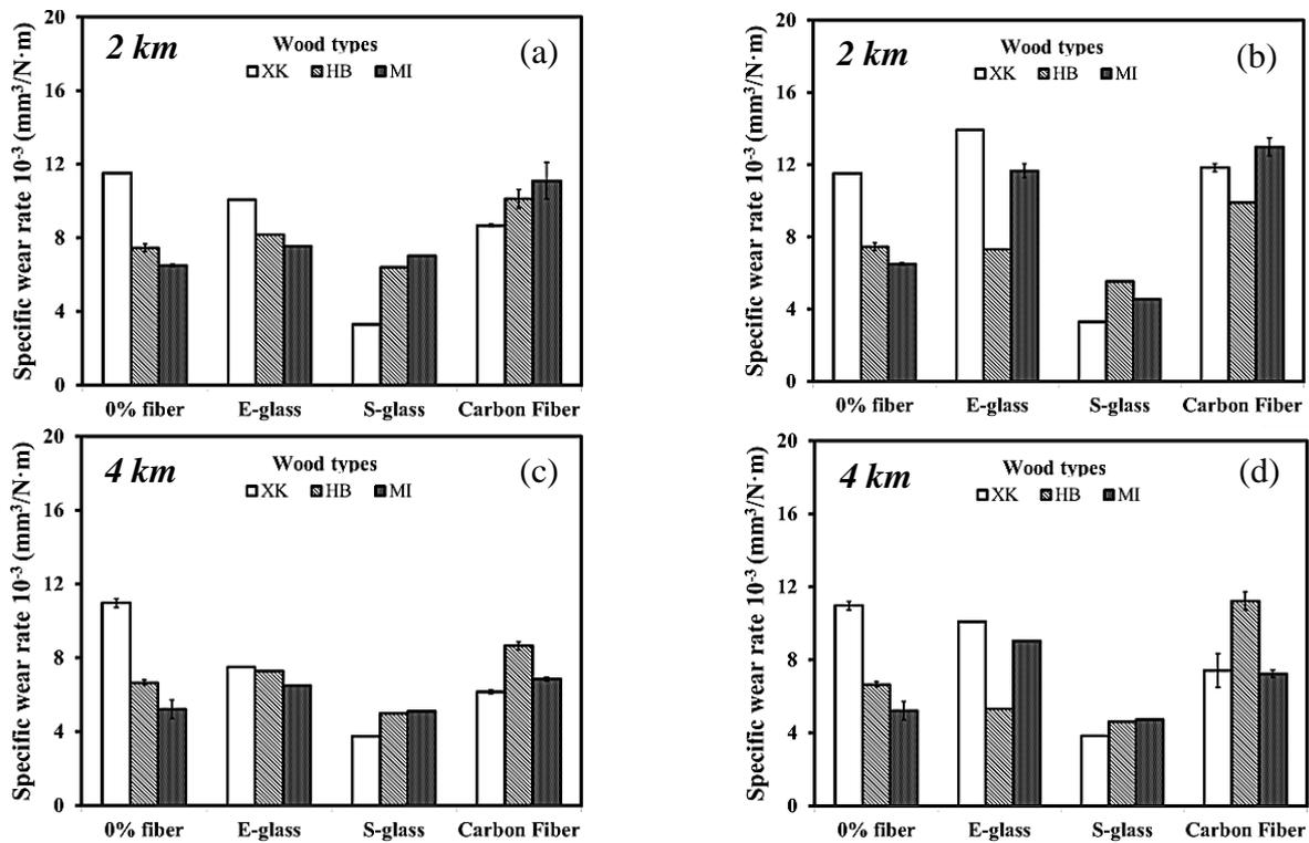
**Figure 3** Specific wear rate of co-reinforced WPVC at sliding distances of 2 and 4 km; where 10 pph of synthetic fiber: (a) and (c) and 20 pph of synthetic fiber: (b) and (d)
