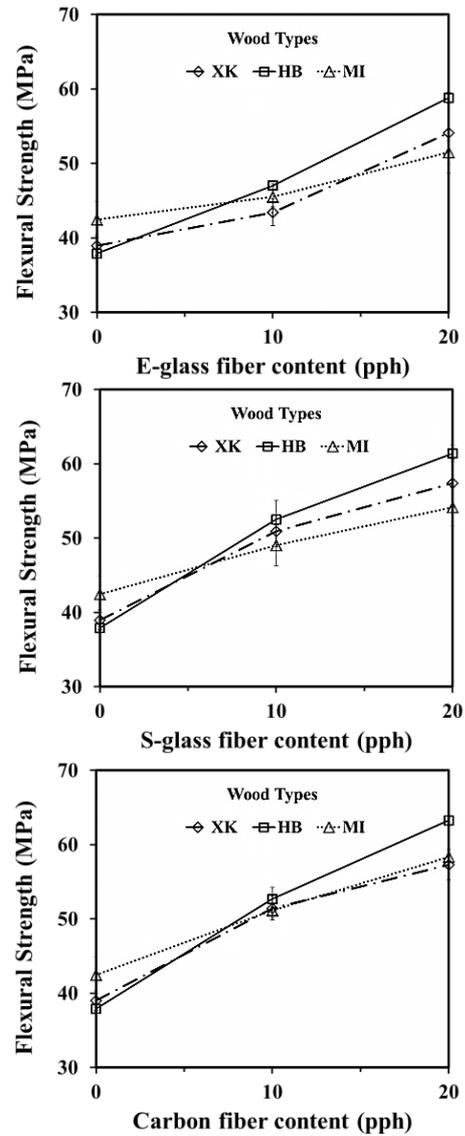
Figure 2 Flexural strength of co-reinforced WPVC
