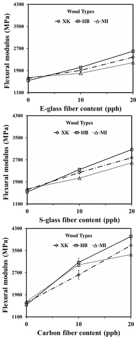
Figure 1 Flexural modulus of co-reinforced WPVC
