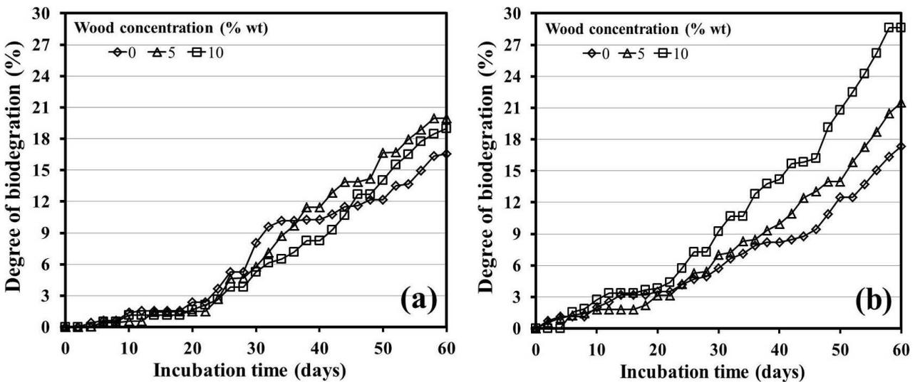
**Figure 3** Degree of biodegradations for PLA without (a) and with 1.5%wt of Zeomic (b) at different wood contents
