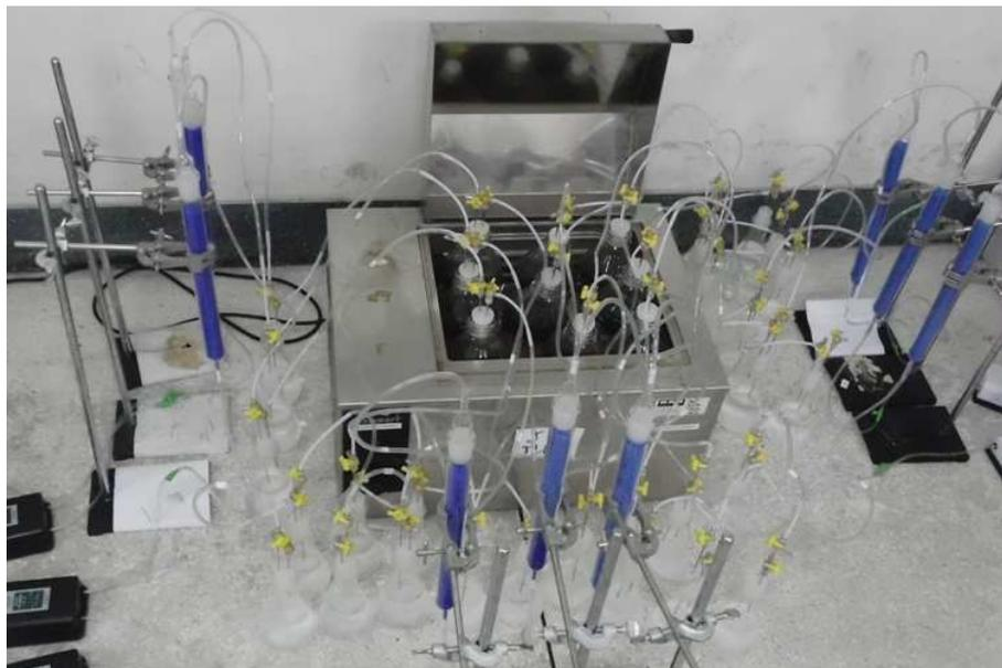
**Figure 1** Set of experimental apparatus for bio-degradation test by soil-composting test as followed by ASTM D5338
