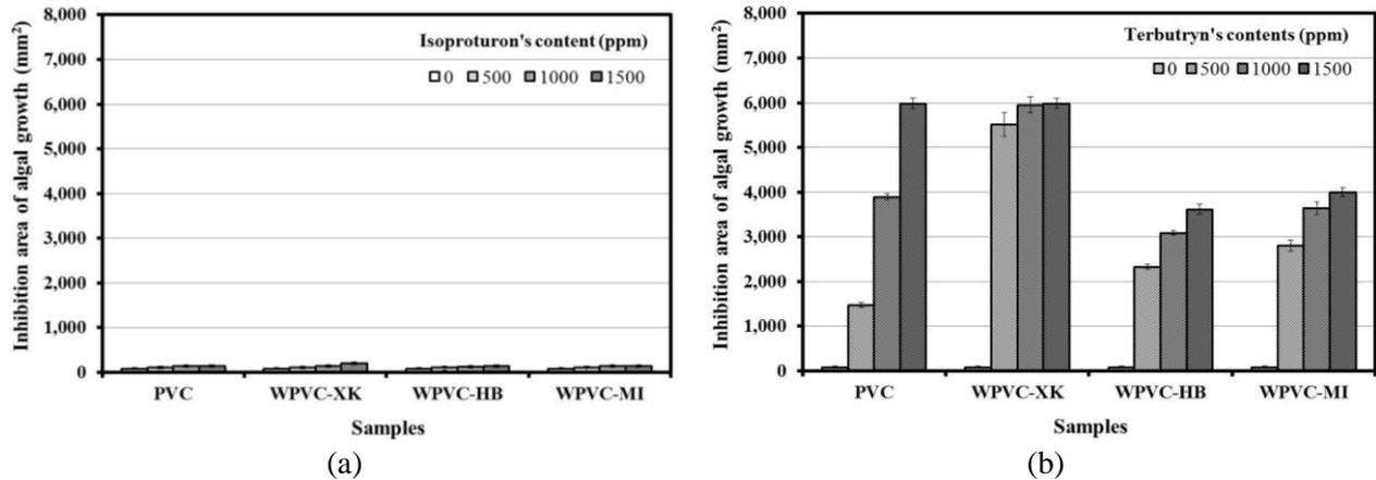
**Figure 1:** Inhibition area of algal growth for PVC and WPVC at different wood types where (a) Isoproturon sample and (b) Terbutryn samples
