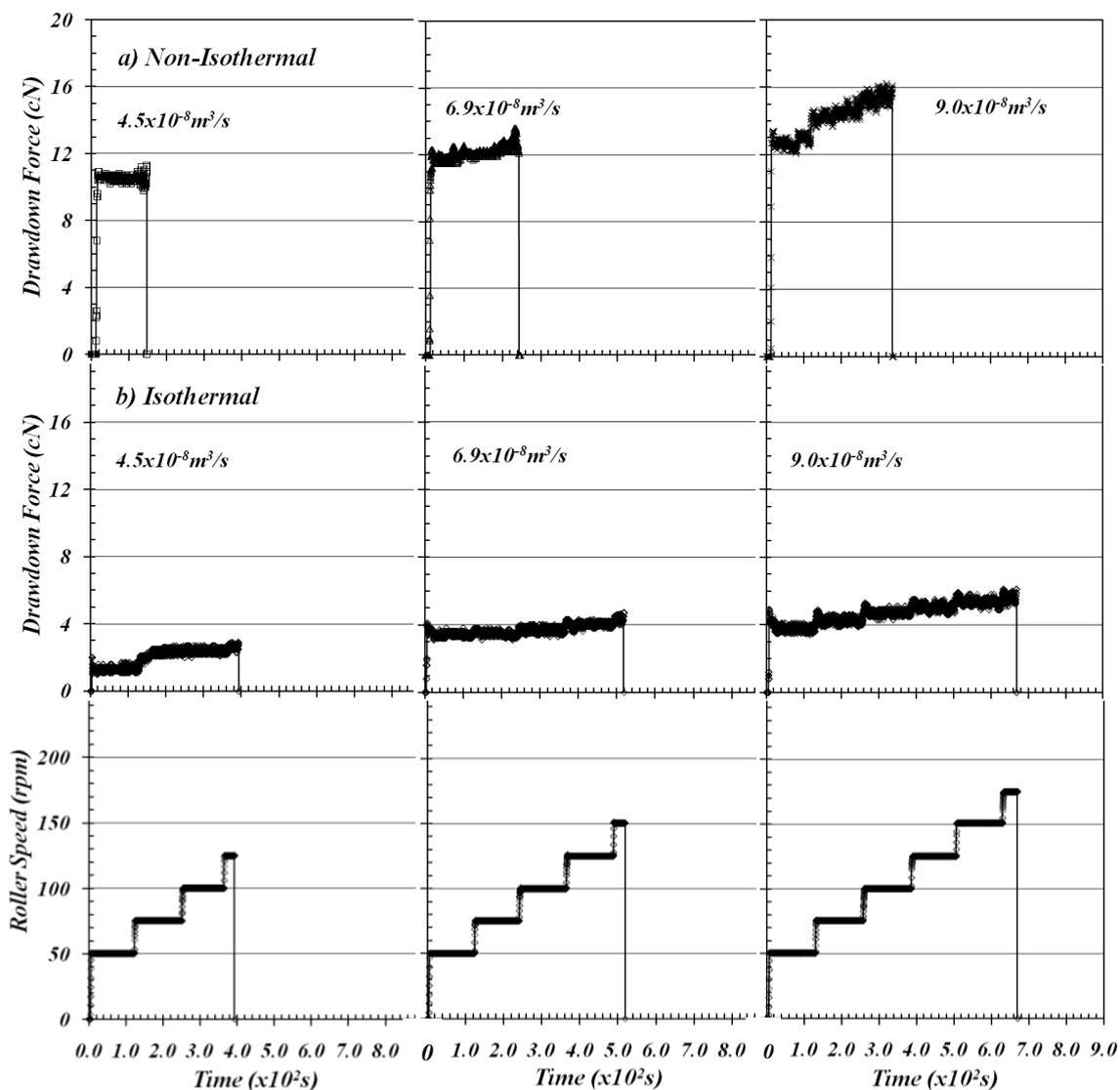
Figure 3. Drawdown force VS time as a function of roller speed for LDPE extrudate filament for three different volumetric flow rates. (a) non-isothermal filament stretching (b) isothermal filament stretching
