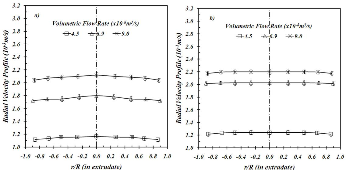
Figure 4. Radial velocity profiles for LDPE filament *without* filament stretching for three difference volumetric flow rates. (a) non-isothermal condition (b) isothermal condition
