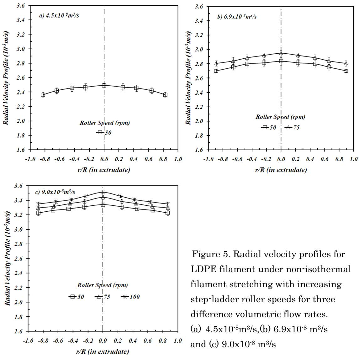
Figure 5. Radial velocity profiles for LDPE filament under non-isothermal filament stretching with increasing step-ladder roller speeds for three difference volumetric flow rates. (a)  $4.5 \times 10^{-8} \text{ m}^3/\text{s}$ , (b)  $6.9 \times 10^{-8} \text{ m}^3/\text{s}$  and (c)  $9.0 \times 10^{-8} \text{ m}^3/\text{s}$
