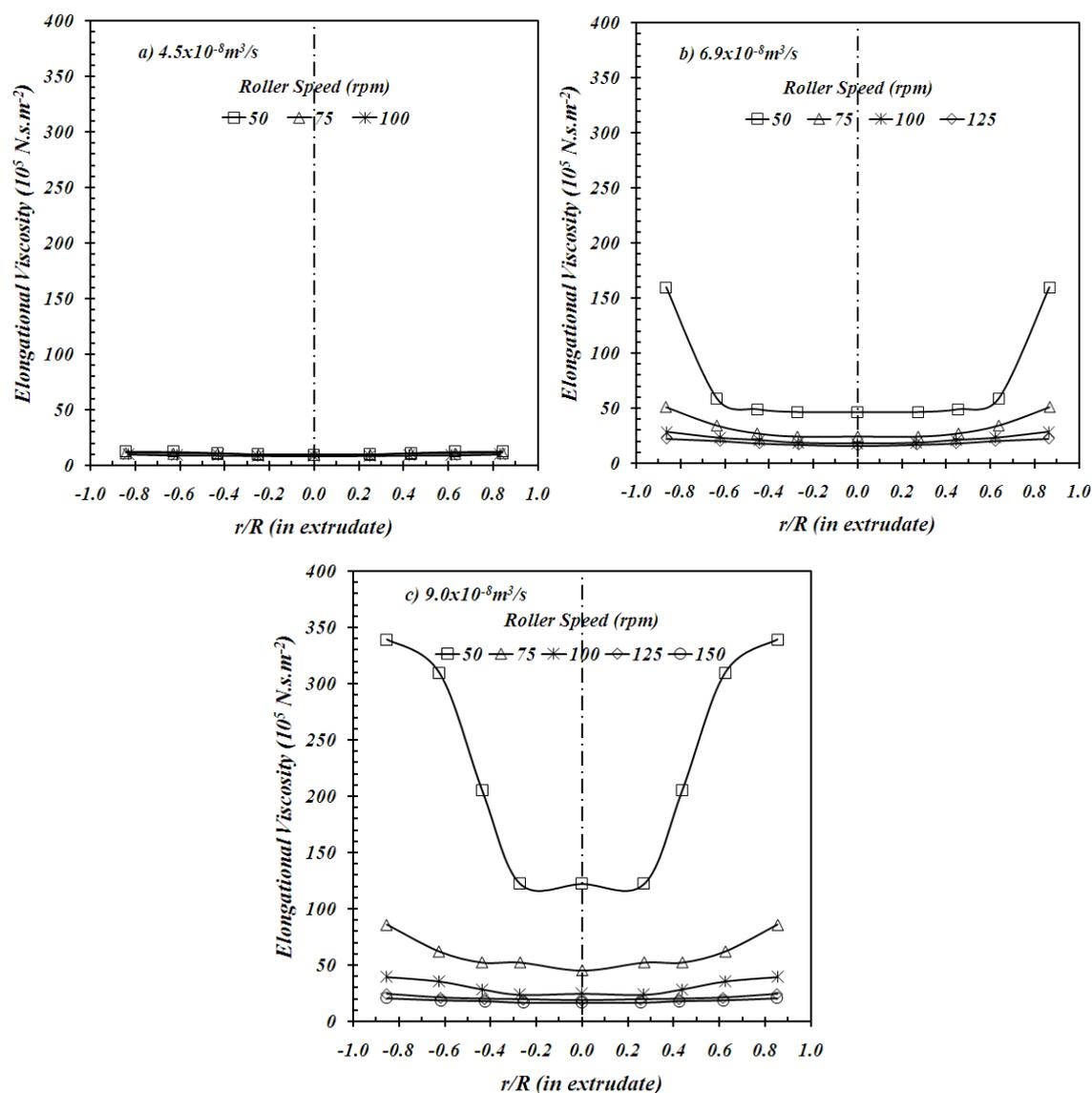
Figure 8. Radial elongational viscosity profiles for LDPE filament under isothermal stretching for three difference volumetric flow rates. (a)  $4.5 \times 10^{-8} \text{ m}^3/\text{s}$ , (b)  $6.9 \times 10^{-8} \text{ m}^3/\text{s}$ , and (c)  $9.0 \times 10^{-8} \text{ m}^3/\text{s}$
