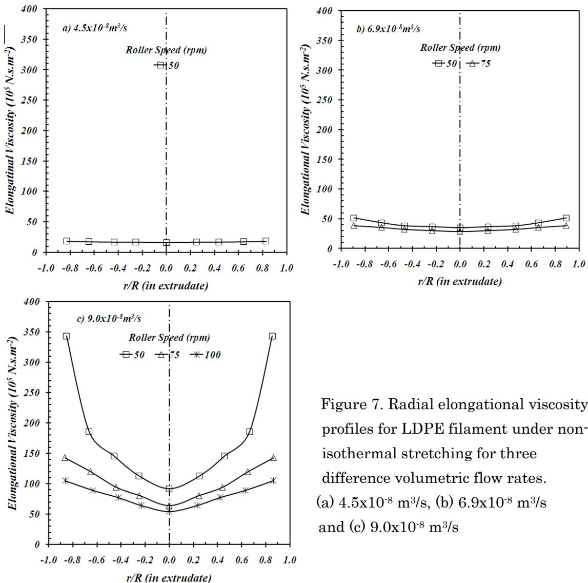
Figure 7. Radial elongational viscosity profiles for LDPE filament under non-isothermal stretching for three difference volumetric flow rates. (a)  $4.5 \times 10^{-8} \text{ m}^3/\text{s}$ , (b)  $6.9 \times 10^{-8} \text{ m}^3/\text{s}$  and (c)  $9.0 \times 10^{-8} \text{ m}^3/\text{s}$
