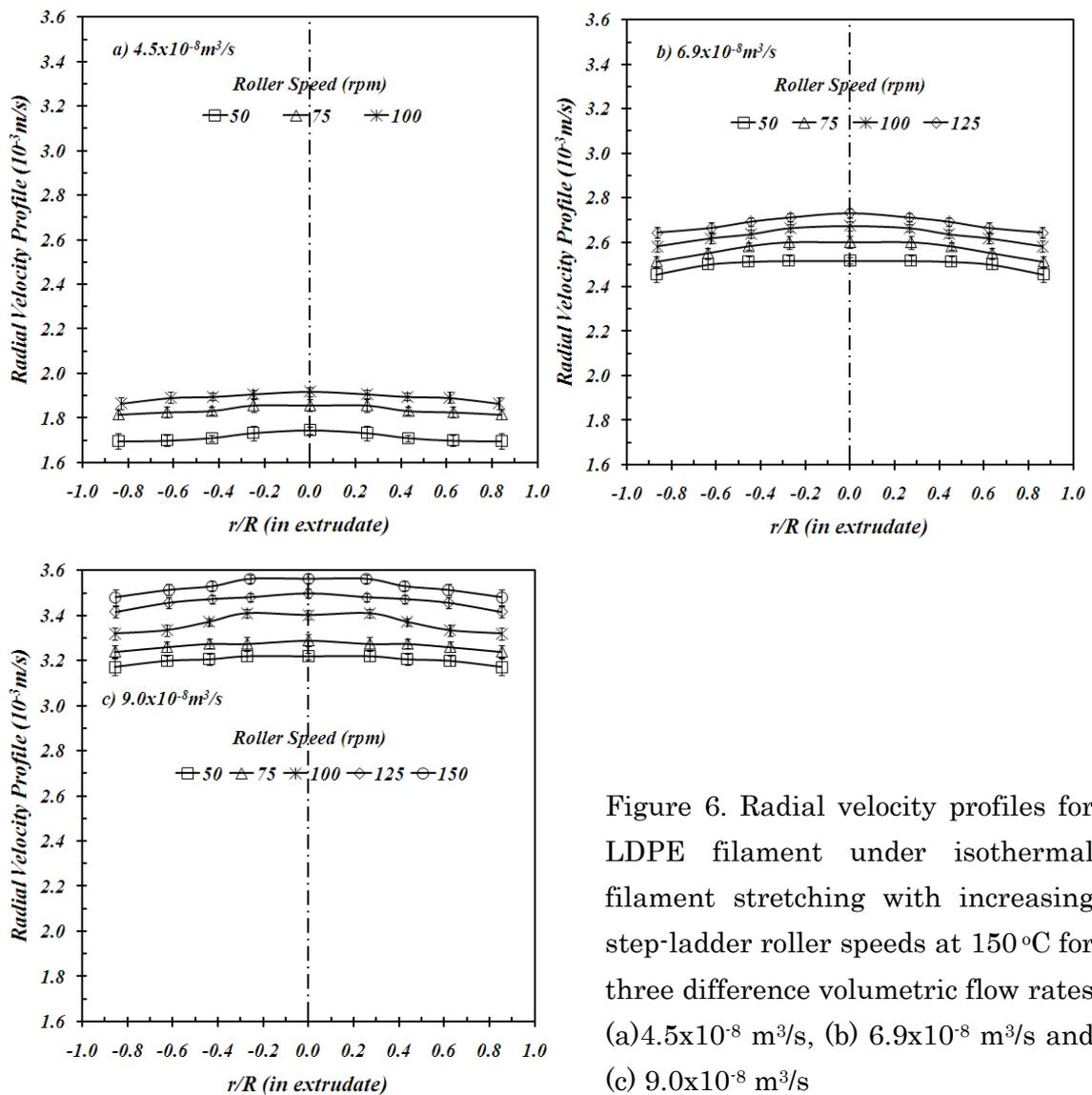
Figure 6. Radial velocity profiles for LDPE filament under isothermal filament stretching with increasing step-ladder roller speeds at 150°C for three difference volumetric flow rates. (a)  $4.5 \times 10^{-8} \text{ m}^3/\text{s}$ , (b)  $6.9 \times 10^{-8} \text{ m}^3/\text{s}$  and (c)  $9.0 \times 10^{-8} \text{ m}^3/\text{s}$
