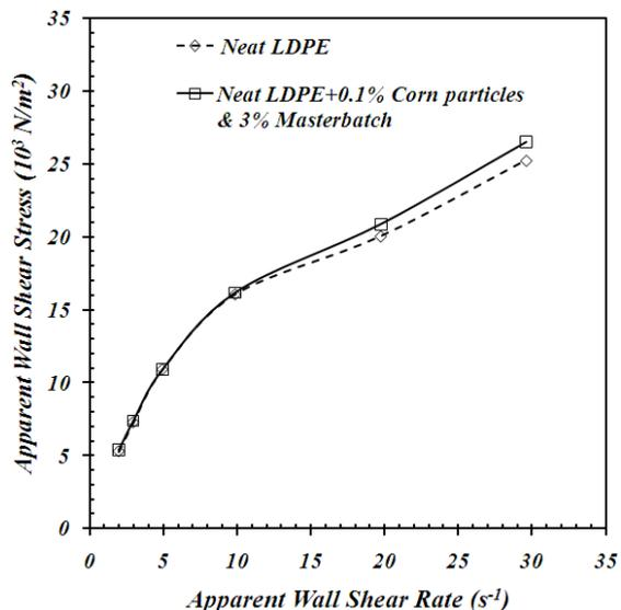
Figure 2. Flow curve of molten LDPE with and without the addition of corn particles and LDPE masterbatch at a die temperature of 150°C
