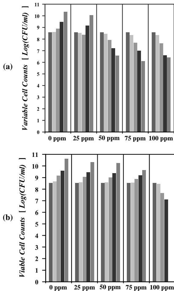
**Figure 3.** Comparison of viable cell count of PE sample having different dosages of nano-silver which were incorporated by spray-coating (a) and dry-blending (b) techniques with contact times 0 min (■), 30min (■), 90 min (■), 150 min (■), and 210 min (■)
