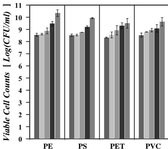
**Figure 1.** Viable *E. coli* colony count for various thermoplastics with different contact times 0 min (■), 30 min (▨), 90 min (▩), 150 min (■), and 210 min (■) without incorporation of nano-silver colloid
