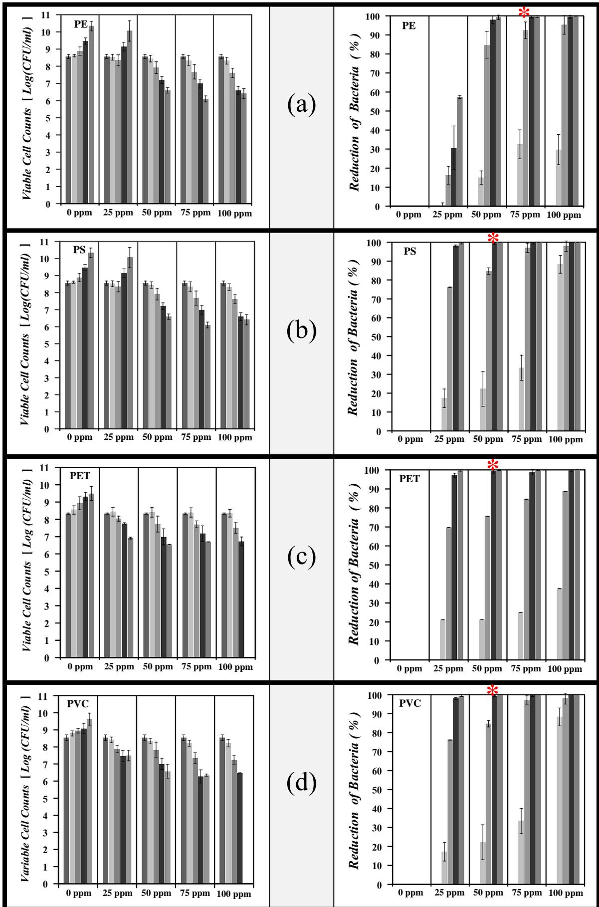
**Figure 2.** Effects of nano-silver content and contact times 0 min (■), 30min (■), 90 min (■), 150 min (■), and 210 min (■) on viable cell count and antibacterial efficacy of nano-silver colloid coated specimens: (a) PE (b) PS (c) PET (d) PVC
