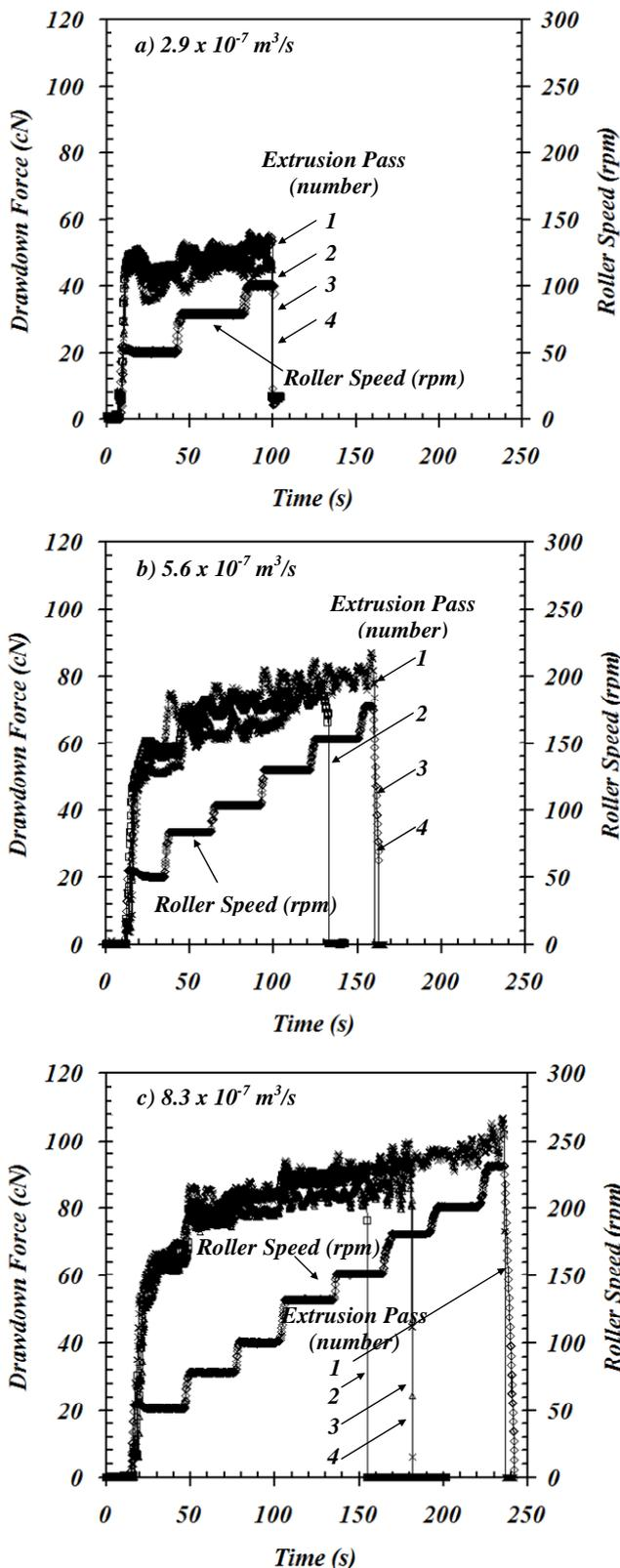
**Fig. 3** Drawdown force as a function of drawdown time at 160 °C of die temperature for a various volumetric flow rates : (a)  $2.9 \times 10^{-7} \text{ m}^3/\text{s}$ , (b)  $5.6 \times 10^{-7} \text{ m}^3/\text{s}$ , (c)  $8.3 \times 10^{-7} \text{ m}^3/\text{s}$
