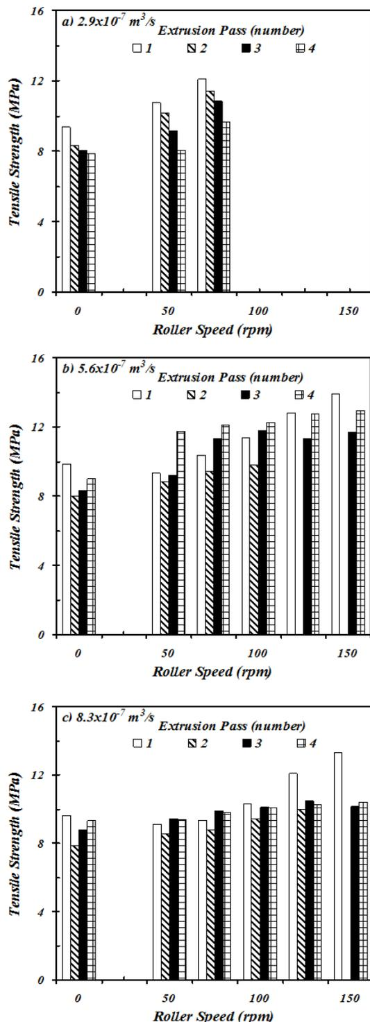
**Fig. 4** Tensile strength as a function of roller speed for a various volumetric flow rate: (a)  $2.9 \times 10^{-7} \text{ m}^3/\text{s}$ , (b)  $5.6 \times 10^{-7} \text{ m}^3/\text{s}$ , (c)  $8.3 \times 10^{-7} \text{ m}^3/\text{s}$
