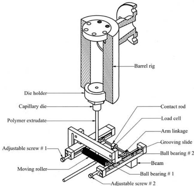
**Fig. 1** An experimental arrangement for melt strength measurement
