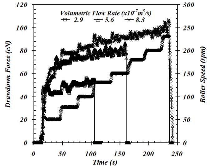
**Fig. 2** Plot of drawdown force as a function of roller speed and drawdown time for three different volumetric flow rates
