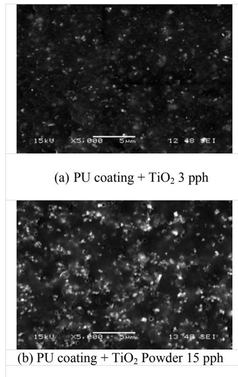
**Figure 2.** SEM micrographs of TiO<sub>2</sub> dispersion on PU coating: (a) 3 pph and (b) 15 pph
