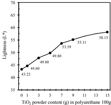
**Figure 3.** The lightness of PU coating on WNR sheet with varying  $TiO_2$  contents
