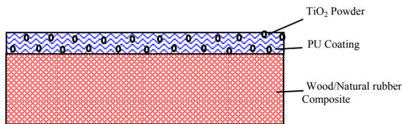
**Figure 1.** WNR layer coated with TiO<sub>2</sub>/PU top-coat
