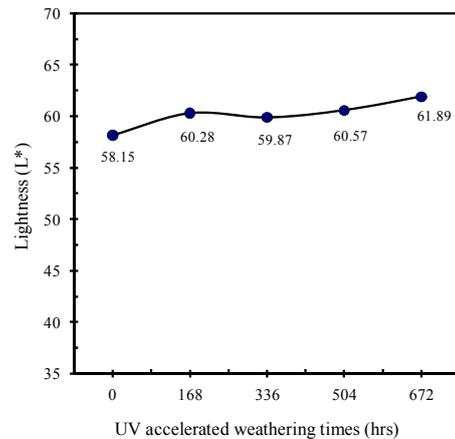
**Figure 4.** The lightness of PU coating on WNR sheet as a function of UV weathering time.
