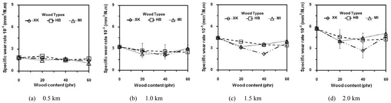
Figure 2 Specific wear rates of WPVC composites without glass fiber reinforcement for different sliding distances
