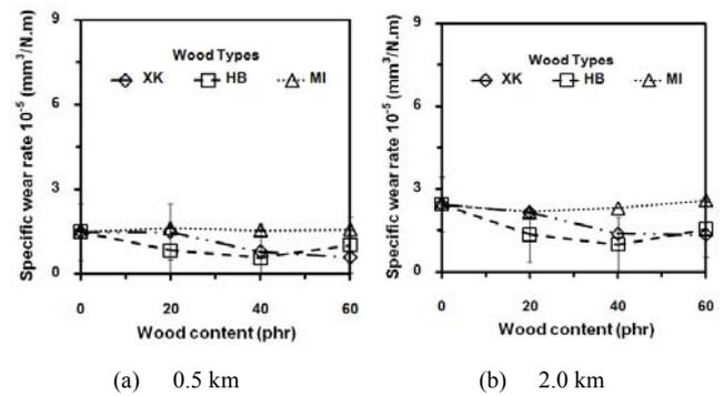
Figure 4 Specific wear rates of WPVC composites with 10 phr glass fiber reinforcement
